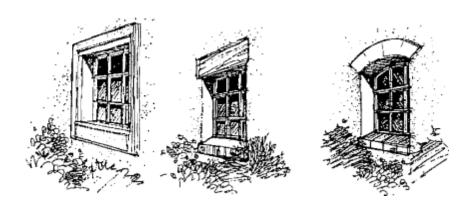
d. Windows- All windows shall be recessed a minimum of 4", or trimmed with a stucco wrapped 2"x 6" or comparable trim detail. Flush windows are not permitted.
