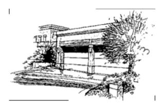
Garage doors shall be sectional metal roll-up. Wood overhead garage doors are not permitted. Garage doors shall be recessed a minimum of 16" from the face of the exterior garage plane, or surround by a 2"x8" pop-out and recessed 12".
