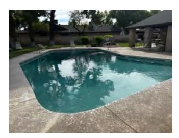
The pool was resurfaced in 4/2010 for \$15,825 and included new trim tile, two (2) new skimmers, two (2) sets of plastic wall steps, two (2) pool lights and two (2) new grab rails.
