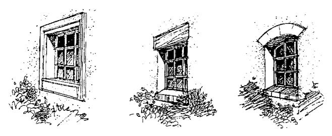
D. Windows - All windows shall be recessed a minimum of 4", or trimmed with a stucco wrapped 2" x 6" or comparable trim detail. Flush windows are not permitted.
